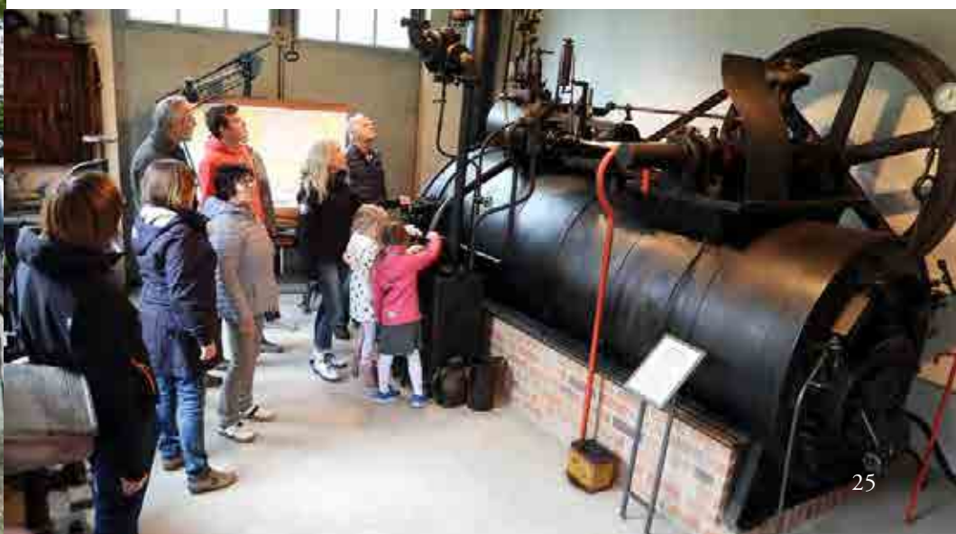
Museum entrance (left), portable steam engine from 1907, for driving the rock crushing plants (right)
