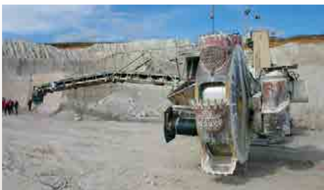
Kaolin is produced using the bucket-wheel excavator SRs 130 in the Kaolin Pit Schleben/ Crellenhain.
